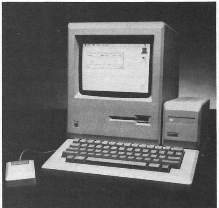
Fig. 12-3. The Paradise Mac 10 hard disk and the Macintosh (courtesy Paradise Systems Inc.).
